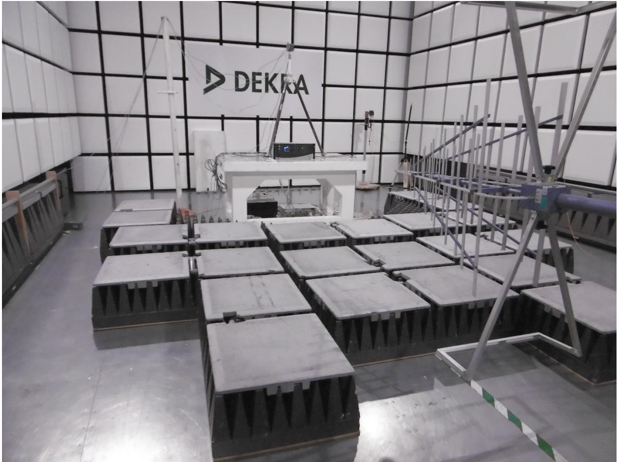
Radiated emission measurement setup 1000 – 6000 MHz.
