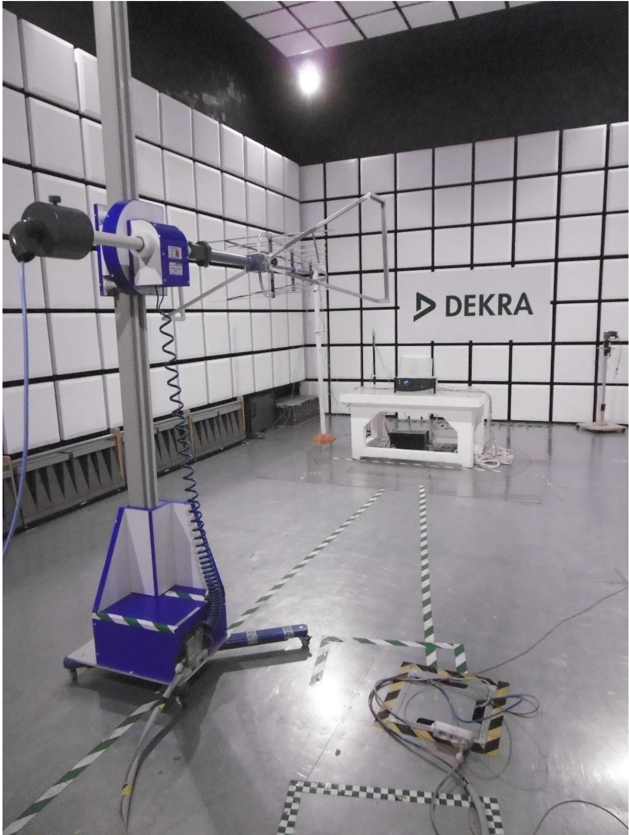
Radiated emission measurement setup 30 – 1000 MHz.
